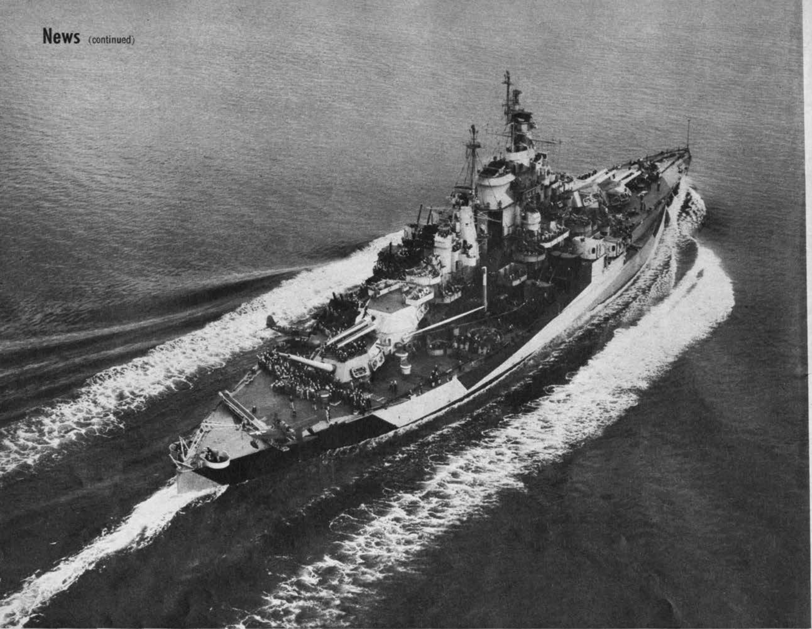
Broad capped stack , characteristic of South Dakota and Tennessee Class battleships, fair into the tower bridge of the rebuilt West Vir-
